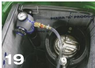
tial corny from my kegerator to do a test run. I gave the corny an hour to settle after moving to avoid foaming. I bled the excess pressure from the keg. I dialed up the  ${\rm CO_2}$  unit until the needle came just off the peg. I pulled the tap into a cup to flush the lines. I grabbed a clean glass. Tipped it under the tap at 45 degrees. I gave the tap a pull . . . and (as seen in photo 20) there was beer!
