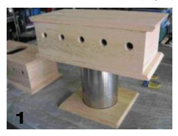
and hoses (as seen in photo 2). The interiors of the draft boxes have been coated with several layers of marine grade polyurethane. Interior joints are sealed with aquarium silicone to waterproof the boxes.
