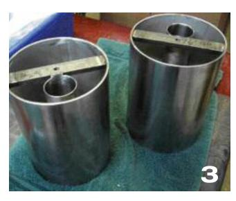
to permit ice to be poured into the top of the draft towers and down into the cylinders to chill the beer line. As the ice melts it drains through the small drilled holes into the red poly tubs. All good theory, but with continual pouring, the beer does not require additional chilling.
