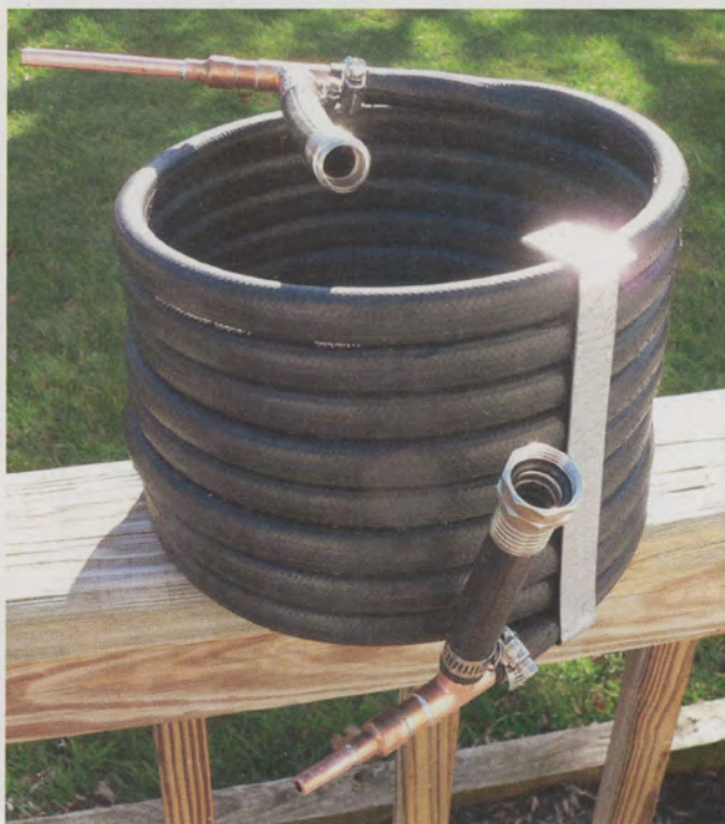
A counterflow wort chiller has one tube inside a second tube. Hot wort travels one way in the inner tube. Cold water travels the opposite direction in the outer tube.
