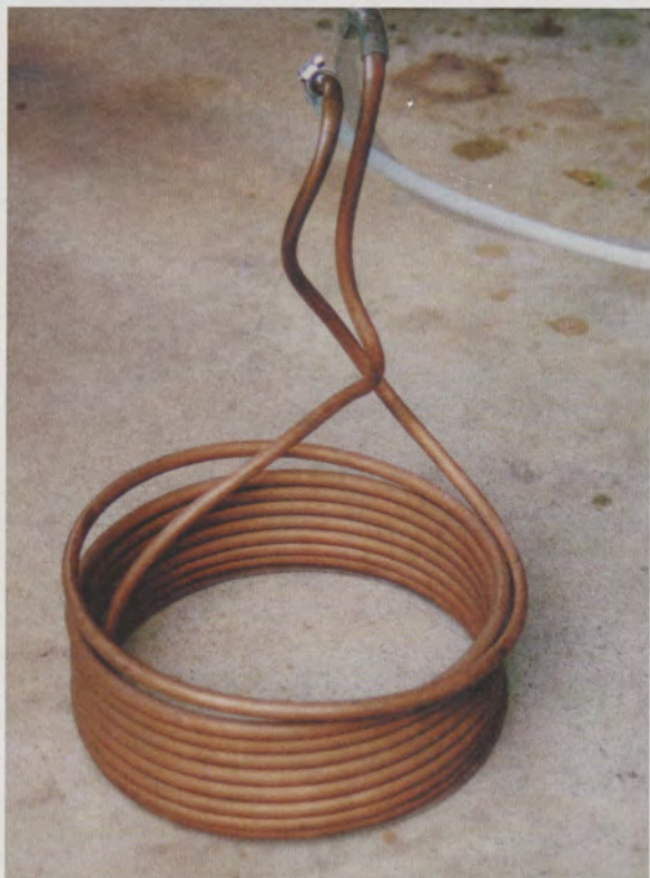
An immersion wort chiller is a metal coil — usually copper — that uses cold water running through the tubing to cool.
