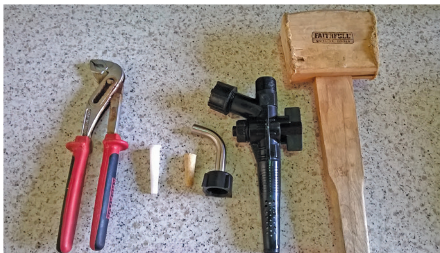
Traditional tools used for serving cask beer: Pliers, hard spile, soft spile, down spout, tap, mallet.
