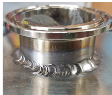
Welding the side exposed to the wort will result in a more sanitary build. Heat tint can be removed with a wire brush while the weld is still hot.
