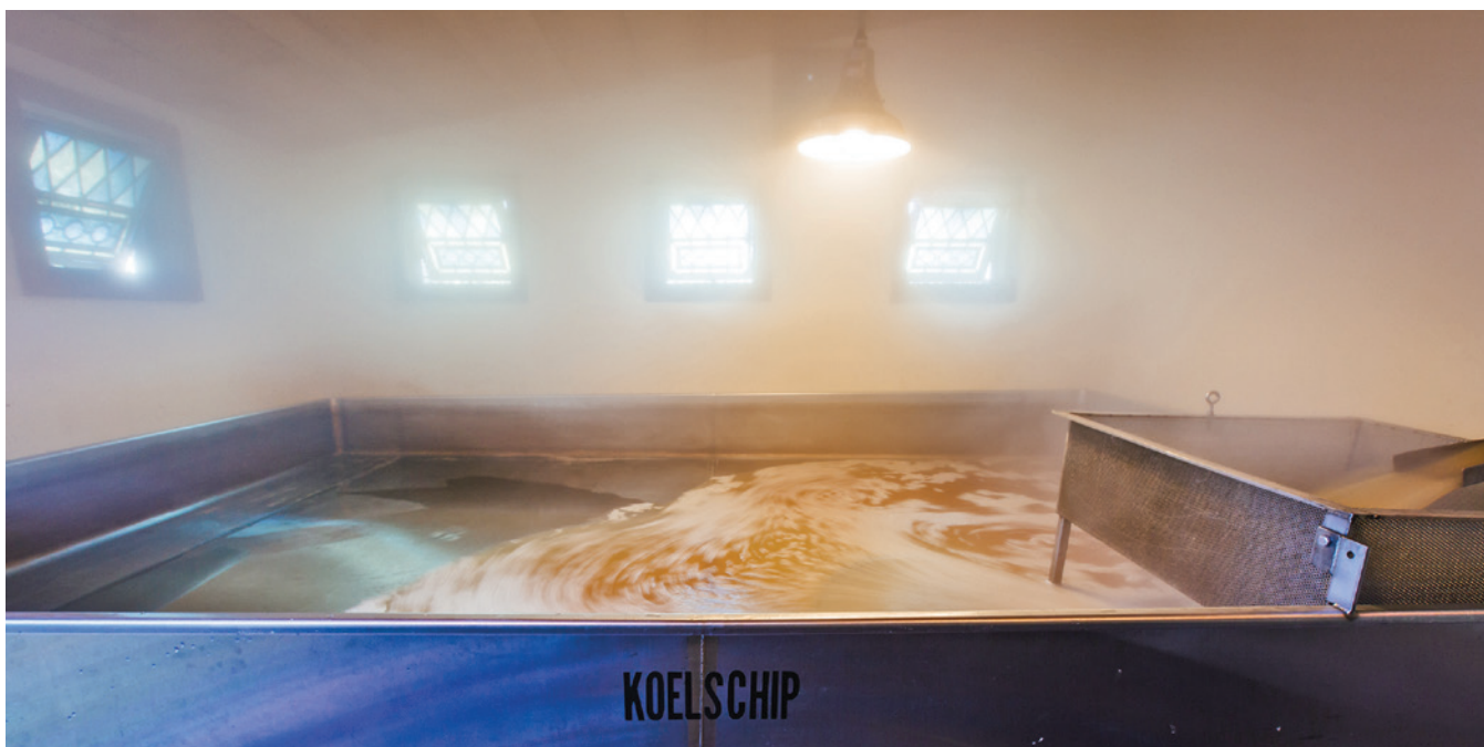
Inspired by the lambic brewers of Belgium, Allagash was the first American brewery to install a coolship in 2007 to create spontaneously fermented beers. Built in a separate space, a fan draws cool evening air as well as native yeast and bacteria through the open windows to cool and inoculate the wort.
