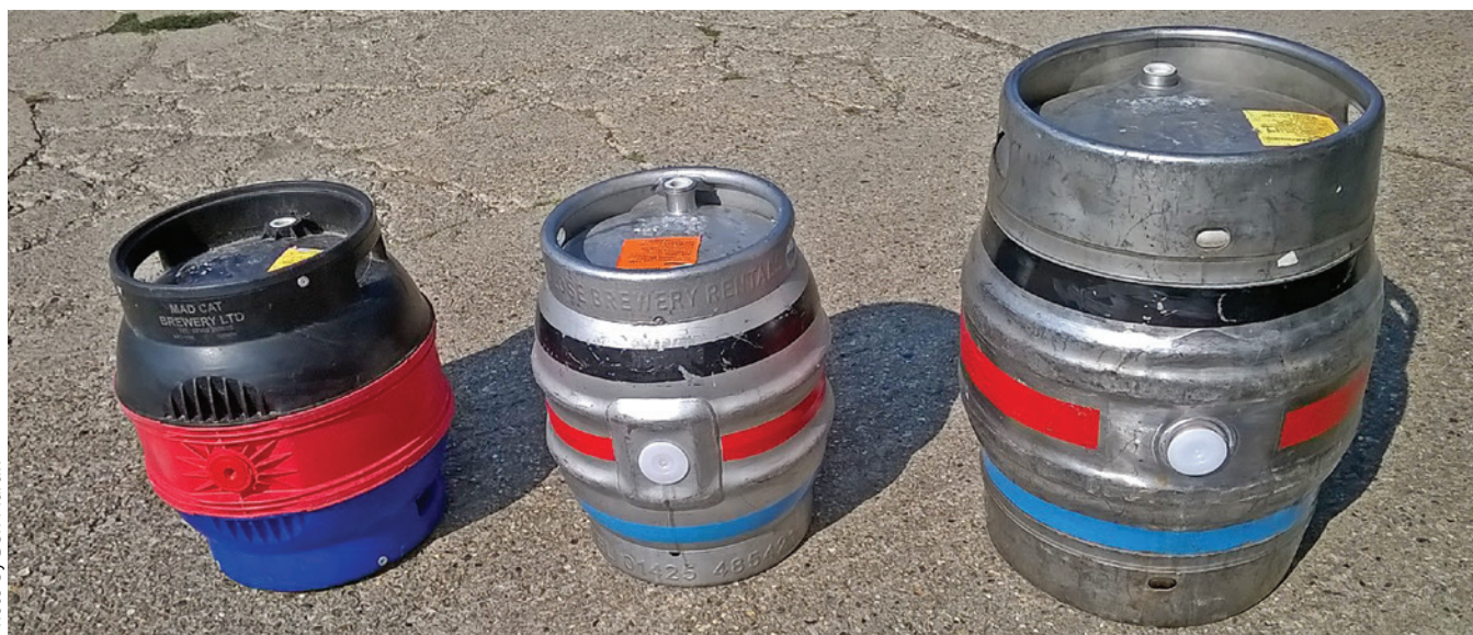
Casks generally come in three sizes (pins, firkins, and kilderkins) and two materials (plastic and steel). Pictured: Plastic firkin, steel firkin, and a steel kilderkin.
