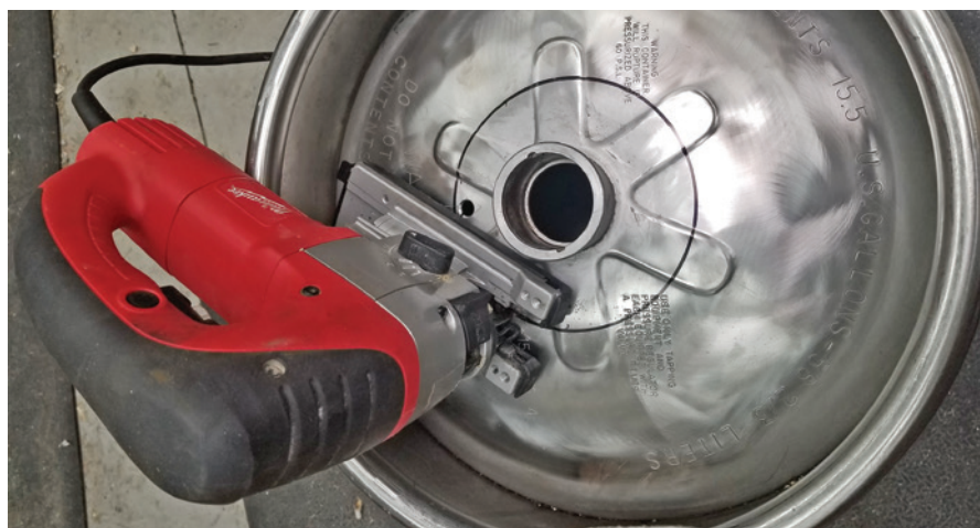
I traced my 6-inch (15-cm) ferrule and used a metal blade in a jigsaw and cutting oil to cut the opening.
