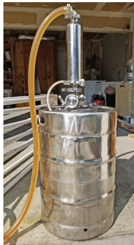
I welded a 1.5-in. (3.75-cm) ferrule in the center on both the inside and outside of the 6-in. (15-cm) ferrule. I attach a strainer on the outside (shown here) when transferring cooled wort into the fermenter to strain out the hot break. When dry hopping I switch the strainer to the inside so I can clean and sanitize the wort strainer and use it to filter out the hops when transferring to kegs.
