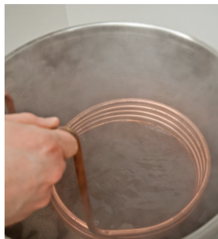
Wort chillers aren't often included in beginning homebrewing kits, although they should be the first piece of equipment to purchase afterwards so wort can be cooled quickly.
