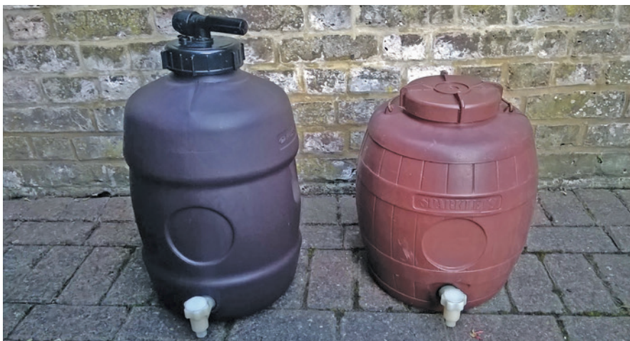
Pressure barrels are popular amongst British homebrewers as CO 2 canisters can help prevent oxidation.
