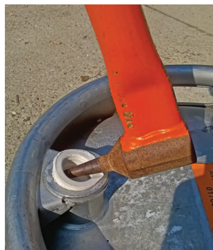
Removing keystone with shive extractor.
