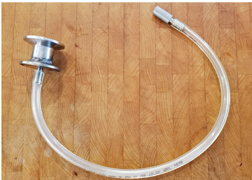
An inexpensive oxygenation/carbonation stone using a ferrule welded to a cap and hose barb.
