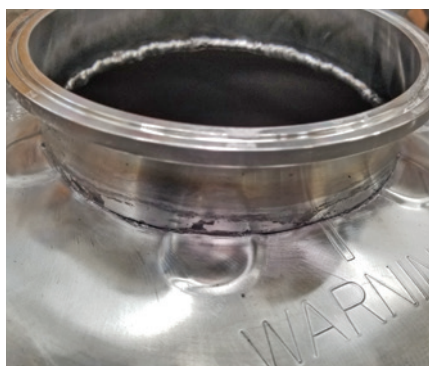
Welding the side exposed to the wort will result in a more sanitary build. Heat tint can be removed with a wire brush while the weld is still hot.
