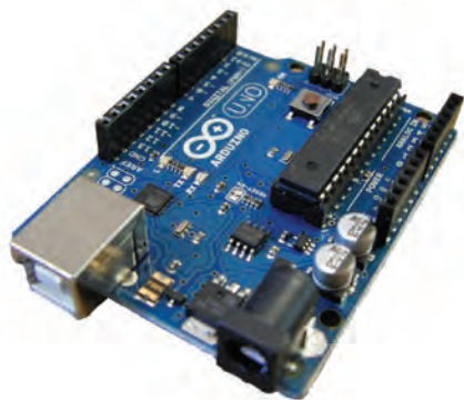
Arduino boards are cheap and popular microcontrollers that homebrewers can use to automate one or several processes in their brewery or cellar.
