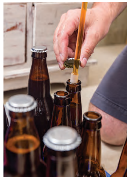
A bottling wand is a handy device to make sure brewers are filling from the bottom to minimize splashing and mixing with air.
