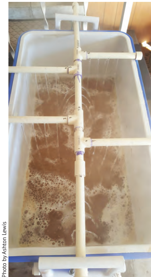
Fly sparging (left) and batch sparging (right) have been shown to have similar extraction efficiencies on the homebrew scale. Make the decision based on your preferences and equipment choices, not efficiency concerns.
