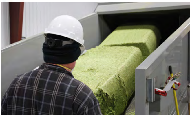
After sorting the hop cones from plant material, the hops are compressed into bales. The bales are split using a bale breaker machine pictured here.
