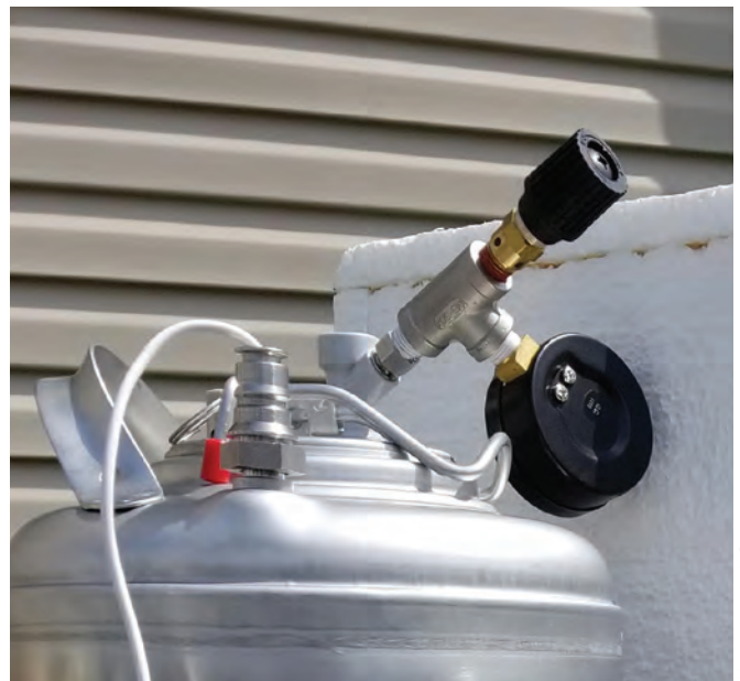
A spunding valve is an effective means to naturally and safely carbonate beer.
