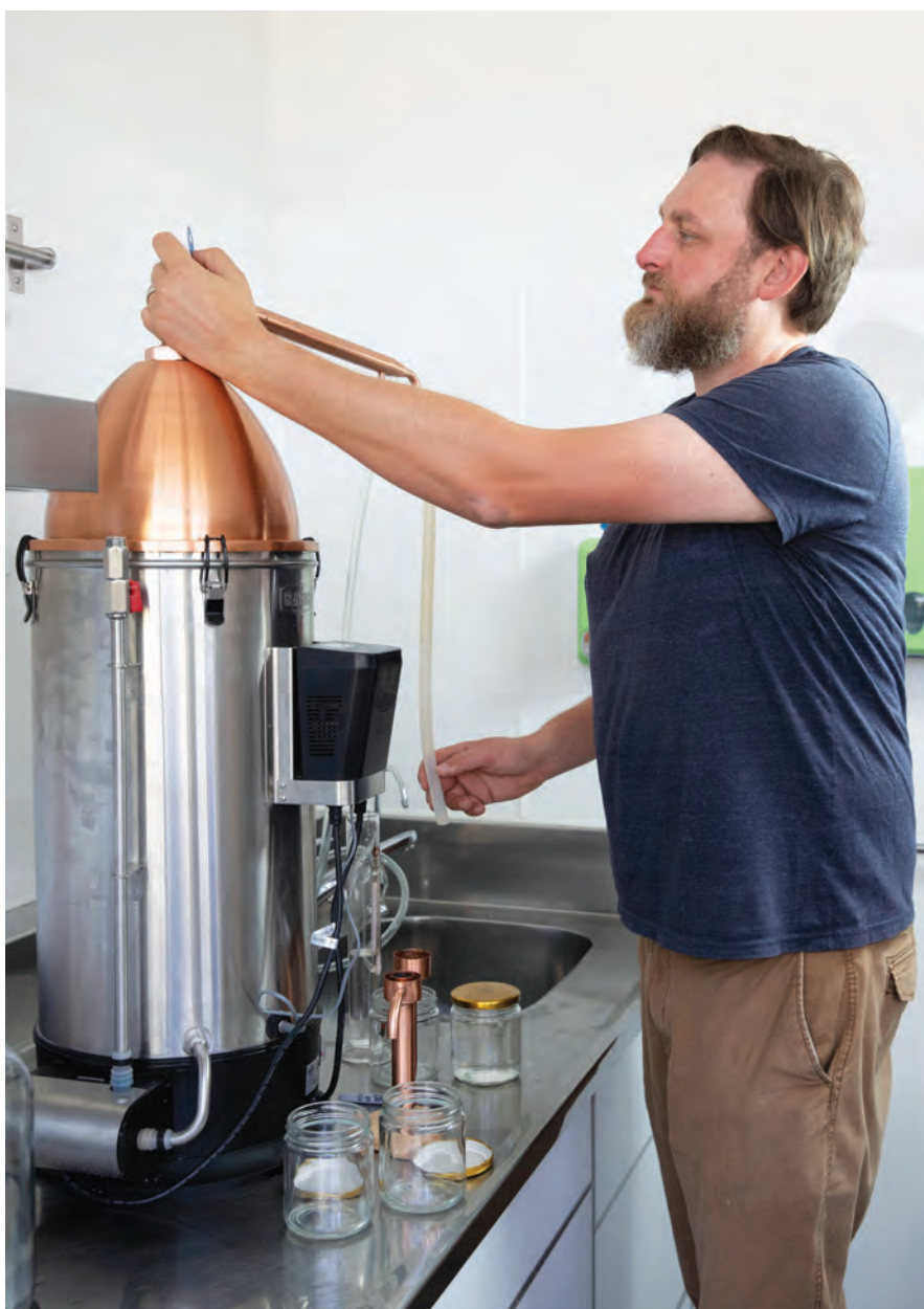
Discard the first 50 mLs out of your still — called the foreshots — which can contain methanol.
