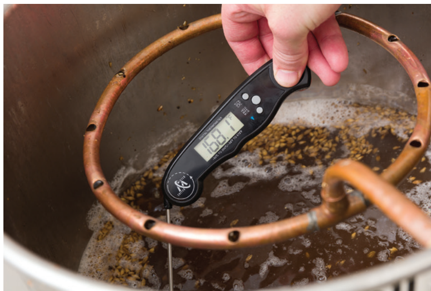
Mashing out around 168 °F (76 °C) will decrease viscosity and increase solubility of extract in the wort—benefits that will help prevent a stuck sparge and improve efficiency.
