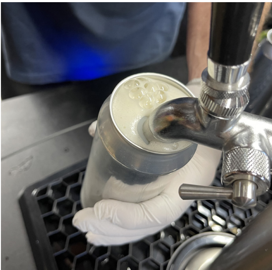
Filling cans with carbonated beer is done in the same way you would fill bottles, including through a line attached to a kegerator faucet. Fill the can high enough that foam rises above the top of the can to minimize oxygen in the can once the lid is sealed in place.
