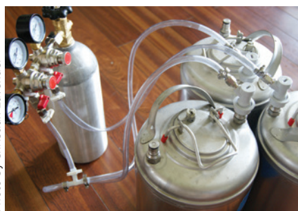
Homebrew draft systems provide users a level of safety in the form of pressure relief valves.
