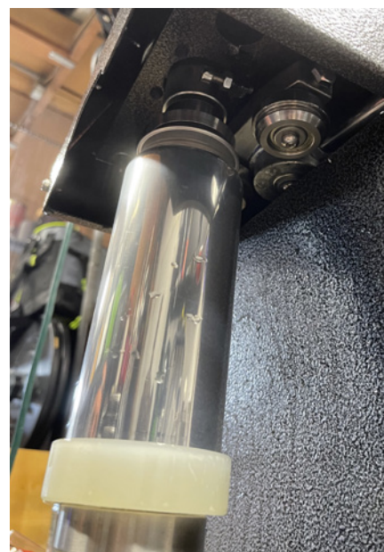
The table raises the filled and loosely capped can against the chuck, which then spins the can as pressure from the rollers seal the lid into place.
