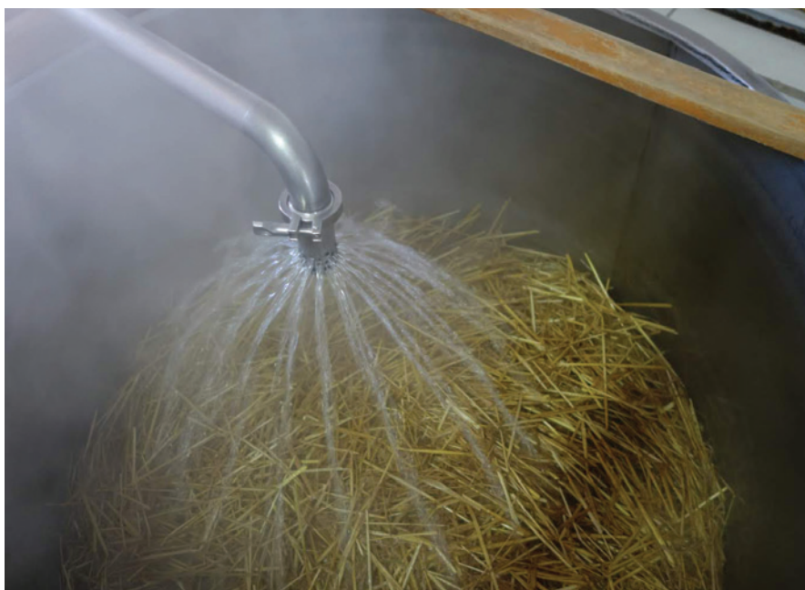
Chicha beer is often filtered using straw in the lauter tun prior to undergoing a mixed fermentation.
