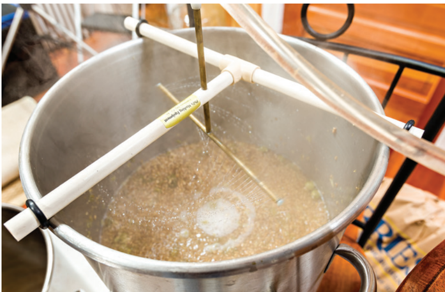
A sparge arm is one way to ensure sparge water is distributed evenly across the top of the entire grain bed without disturbing the grain itself.
