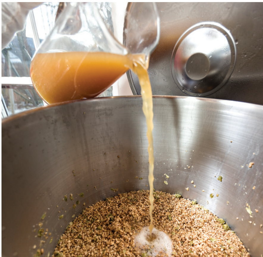
Performing a vorlauf step, where about 10% of the wort is drawn off and then poured back over the grains, allows the grain bed to set and also helps filter out small bits of grain before running the remainder of the wort to the boil kettle.
