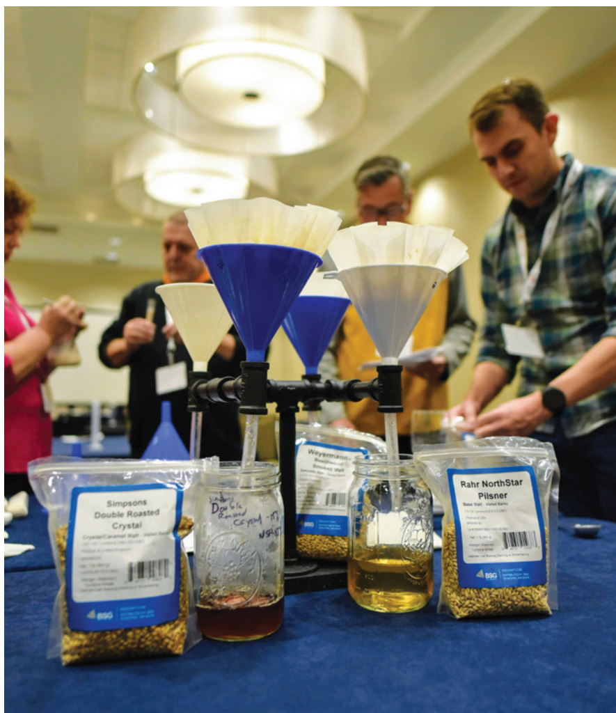
Steeped grain using the ASBC hot steep method is a good way to evaluate malt flavors.
