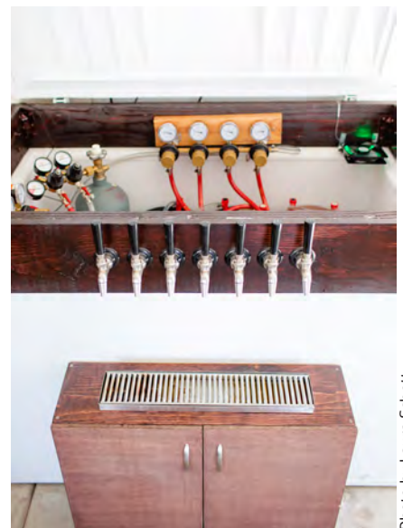
Multiple regulators allow brewers to carbonate and maintain kegs in their kegerator at different levels while also utilizing CO 2 as tool.
