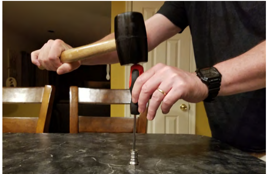
If the keg you're using has "permanent" poppets you will need to force the liquid post's poppet out to allow the temperature controller's probe through. This can be done by placing the poppet upright and tapping the head of the poppet with a screwdriver tip and a mallet.
