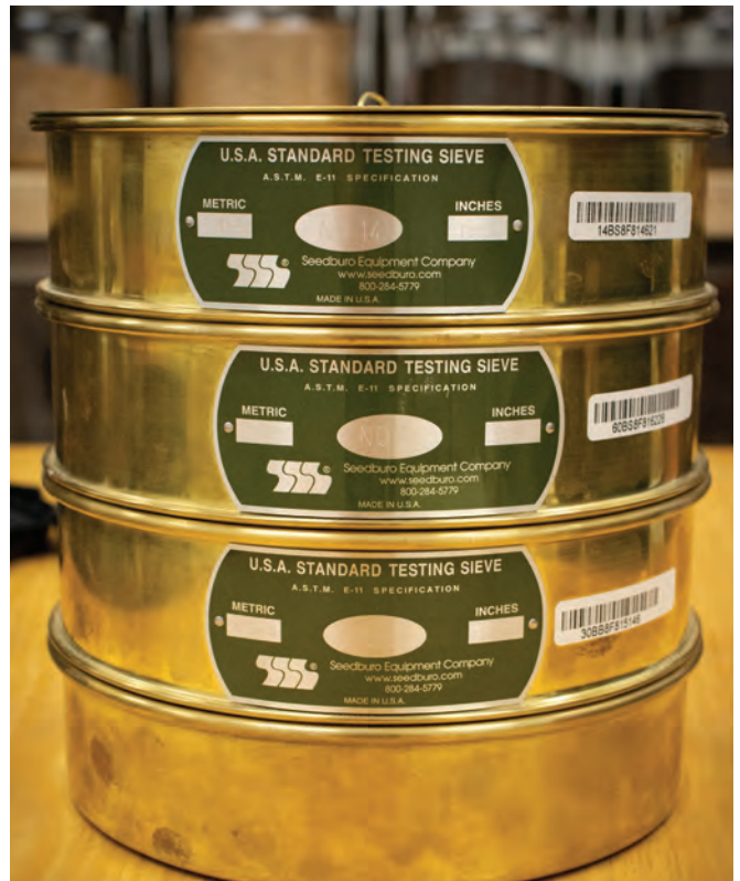
A US standard testing sieve has three layers with different-sized screens, from largest gaps to smallest top to bottom, and a pan on the bottom. By methodically shaking the sieves you can calculate the percent of coarse, standard, and extra fine crush results from your mill gap setting.
