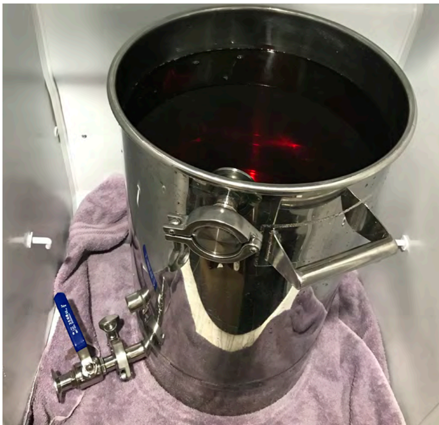
Making ice cider requires freezing the apple juice. In my experience, it can take a week or more to freeze 10 gallons (38 L) solid. Doing this in a vessel with an outlet at the bottom makes collecting the thawed juice easier.
