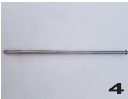
Top to bottom, turning a dip tube into a thermowell: 1. Cut the dip tube to about half the length of your keg and insert the stainless steel plug into the tube. 2. Solder or TIG weld the plug into the new end. 3. Polish the welded/soldered end clean using a file, sandpaper, and finishing with a fine Scotch-Brite pad. 4. Your new thermowell.
