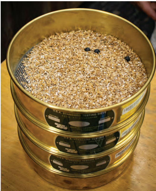
A US standard testing sieve has three layers with different-sized screens, from largest gaps to smallest top to bottom, and a pan on the bottom. By methodically shaking the sieves you can calculate the percent of coarse, standard, and extra fine crush results from your mill gap setting.
