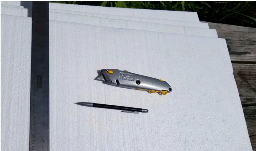
Repeated light scoring with a sharp blade, followed by “pushing” down with the knife rather than “dragging” it, helps to cut through without fragmenting the polystyrene foam sheets.
