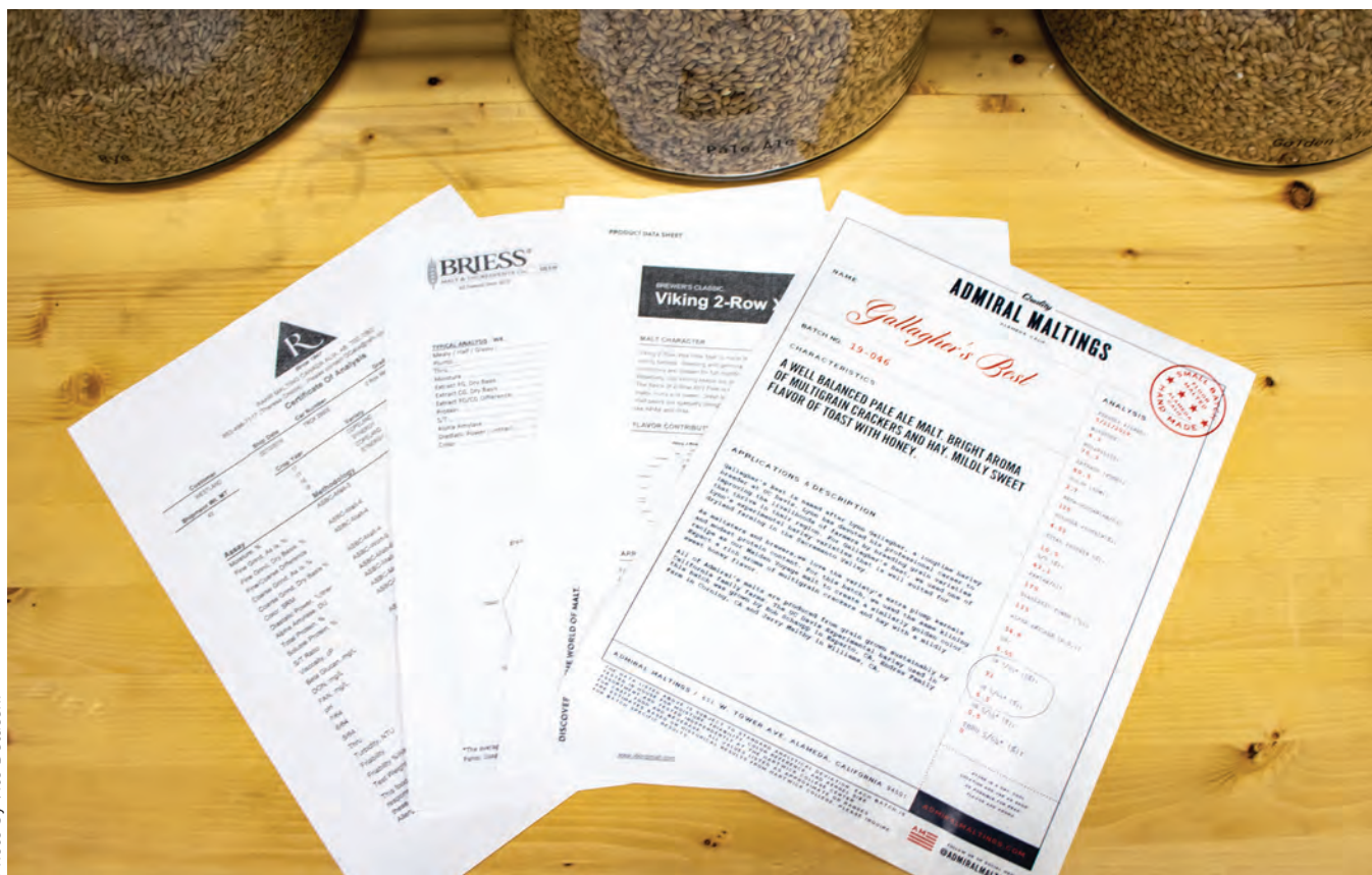
Malt analysis sheets, also called Certificates of Analysis (COAs), should be available from every maltster and contain a lot of useful information about the malt you are using. In terms of the gap settings when crushing, friability and lot assortment are both critical.
