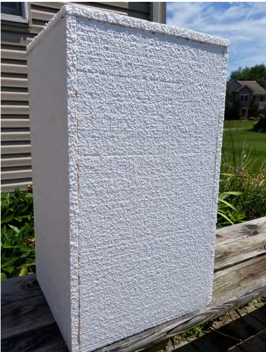
Use construction adhesive to join the sides and then top of your foam insulation enclosure. This insulated box will help maintain a constant temperature for your Lacto “kettle” keg.
