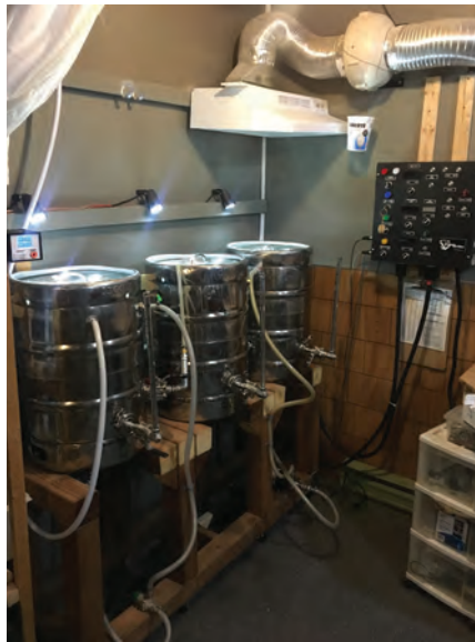
Single-tier, bottom-drained, electric HERMS system designed and engineered by a gearhead, for a gearhead.
