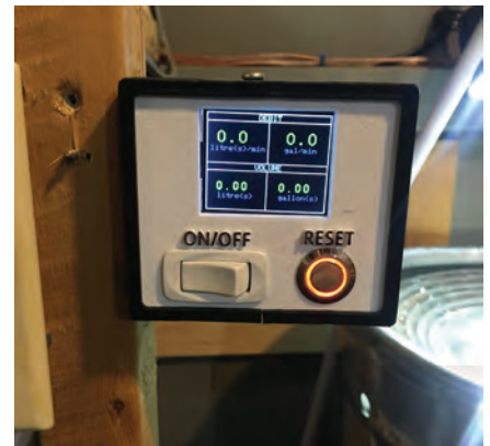
A water flow meter allows precise and accurate measurements of the water coming into the hot liquor tank.
