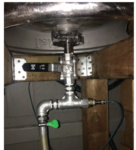
Draining the wort from the bottom of the keggles allows every drop to be collected from the mash, allowing for a highly efficient system.
