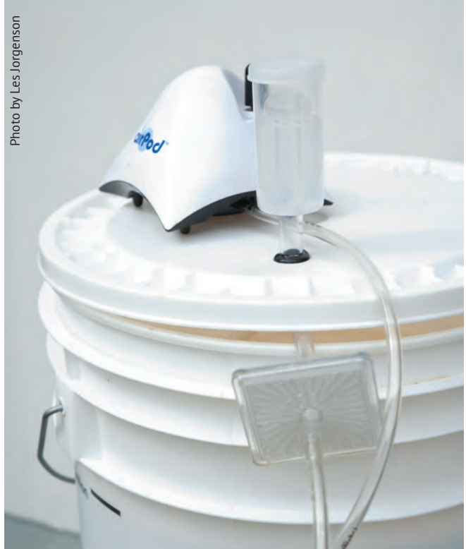
Aerating the wort with an aquarium pump, filter, and diffusion stone is a cost-effective alternative to pure oxygen since it provides a level of oxygen ideal for most all situations.
