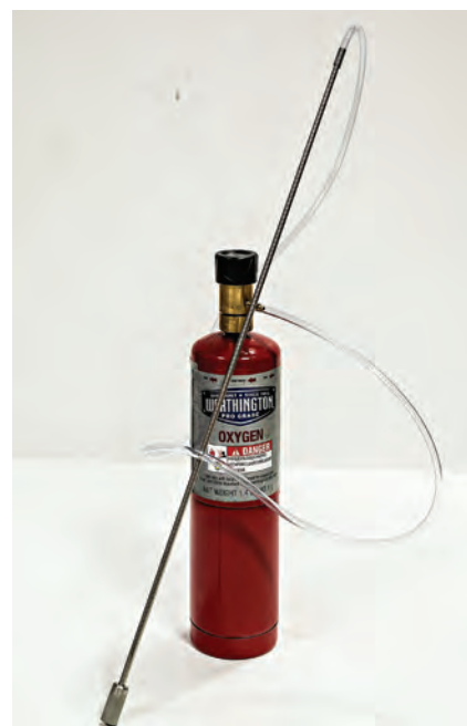
Oxygenation involves injecting pure oxygen into wort, best done with the aid of a regulator, filter, and diffusion stone.
