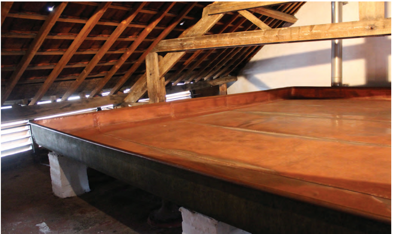
The coolship at Cantillon, where hot wort is pumped to cool and pick up ambient yeast and microbial flora in the air of Brussels, Belgium.
