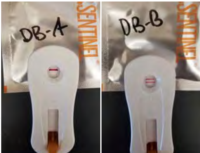
(Left) negative PCR test, no STA1 detected. (Right) positive PCR test, STA1 gene detected above threshold.
