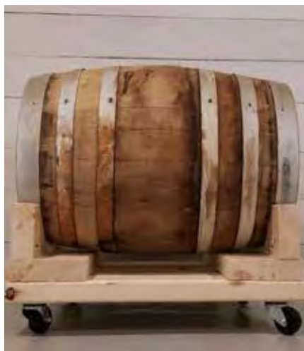
Oak barrels are heavy and awkward to move around when full. A barrel cradle built on caster wheels is an easy solution to this problem.
