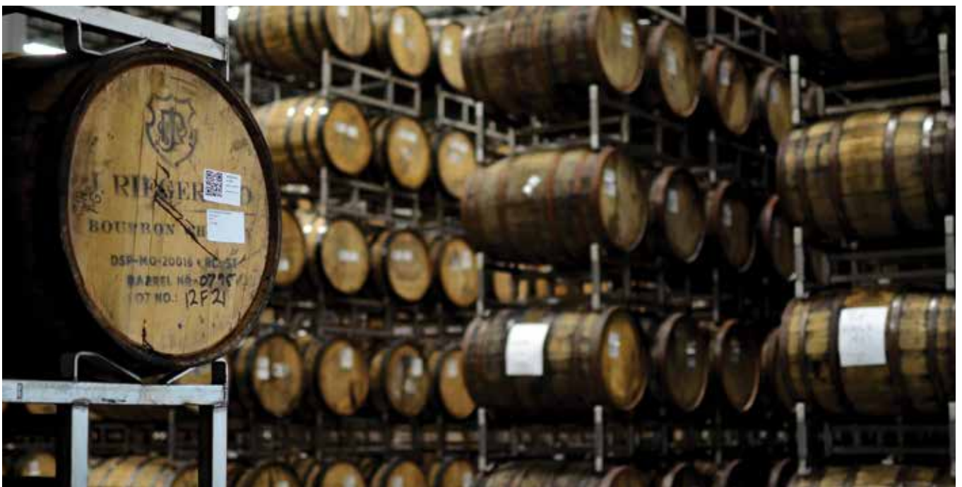
Boulevard's mixed-fermentation and barrel program includes about 5,000 used oak barrels, four vertical foudres, one horizontal foudre, and its own bottling line. Clean beer is transported from the brewhouse to the off-site facility where it is allowed time to age with wild cultures.
