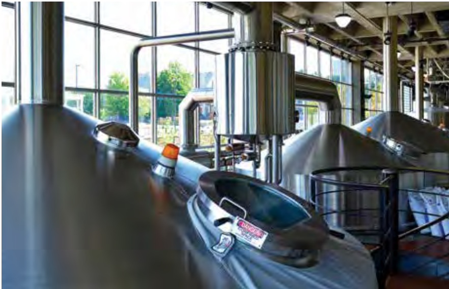
Brewery II is a 4-vessel, 150-barrel brewhouse commissioned by world-renowned German equipment supplier Krones-Steinecker in 2006.
