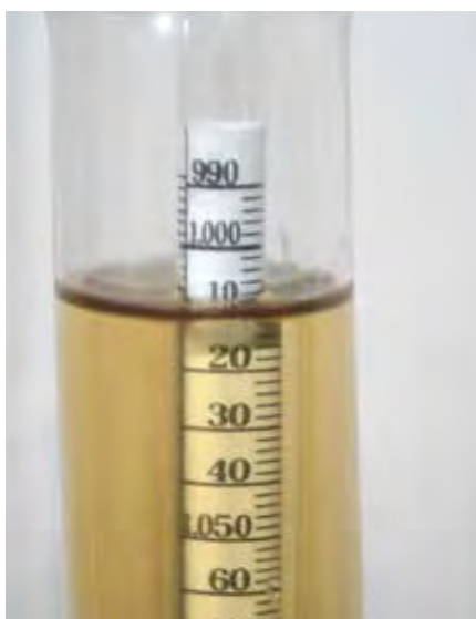
Some sugar is consumed during the kettle-souring phase by Lactobacillus , creating lactic acid. A hydrometer reading can tell you about how much.
