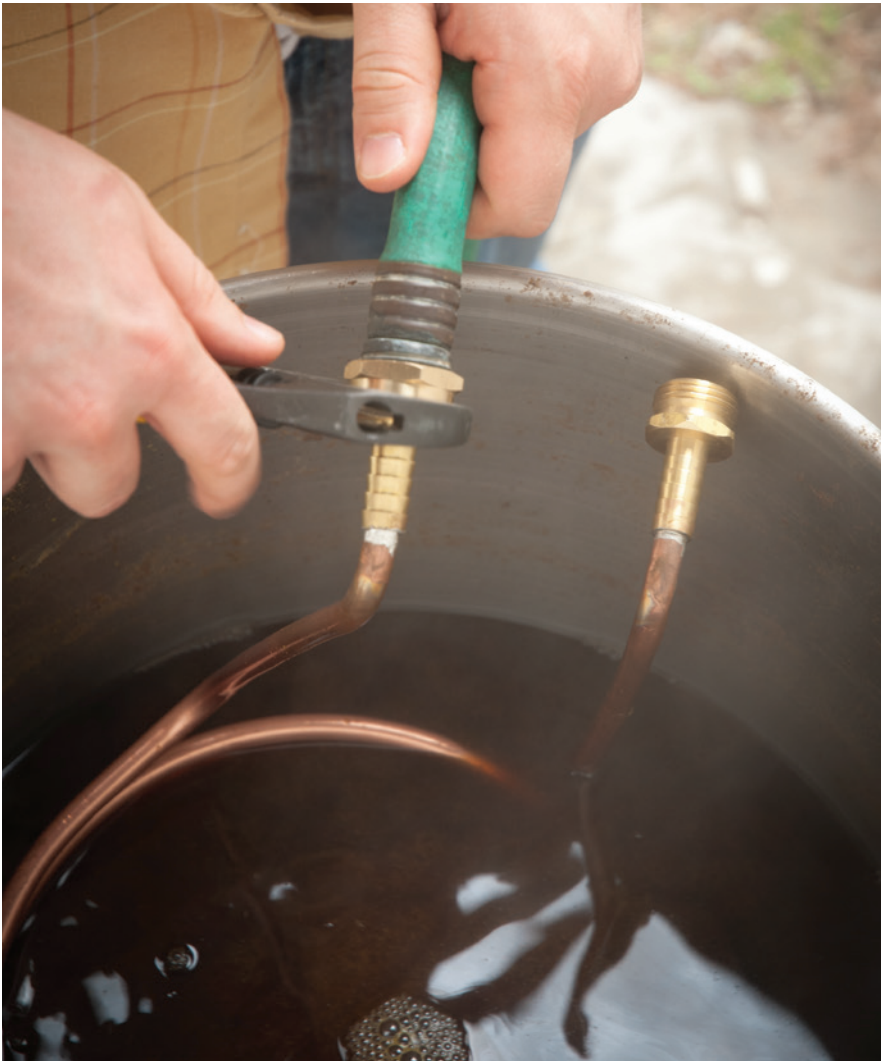
Circulating cold water through an immersion wort chiller is an easy way to get your hot wort down to fermentation temperature post-boil.
