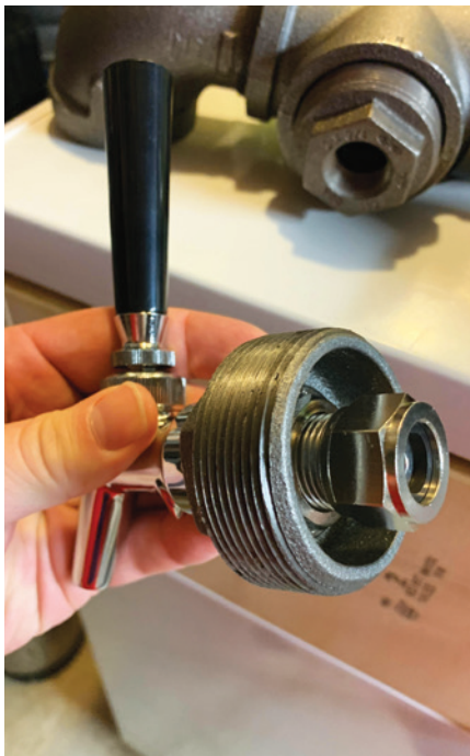
Here is a look at what the reducer bushing and beer shank look like on the back end.
