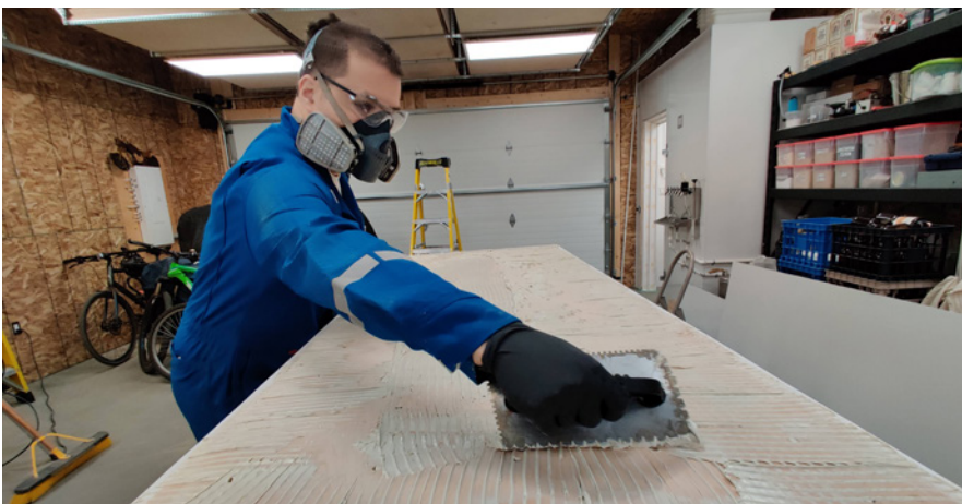
Three layers of maple plywood with foam insulation between each and the plastic shell glued on with a water-based adhesive make up the body of the triple-sealed door.
