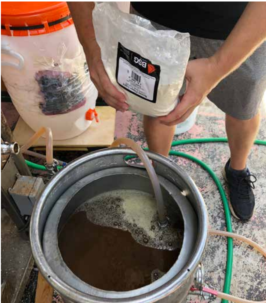
Adding dried malt extract (DME) is another method to increase the original gravity for a batch. I add it during the whirlpool after draining off the wort for the lower gravity batches.
