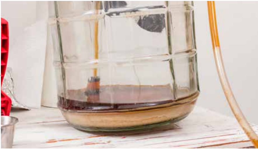
One of the largest reasons for fermenter losses is due to the compacted yeast slurry on the bottom of the fermenter. Yeast slurries are about 25% yeast solids, and the remainder is beer loss.
