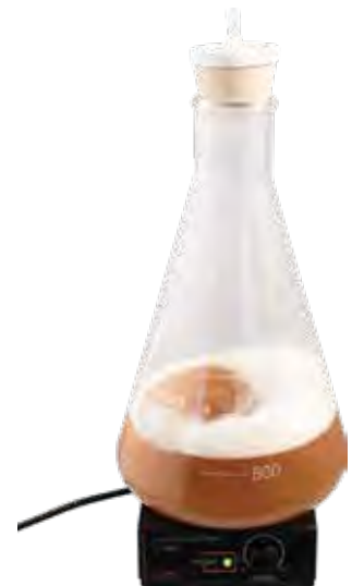
A 2-L flask sealed with a sterile filter in the bung allows gases to flow both ways from a flask without compromising the sterile nature of the closed environment.
