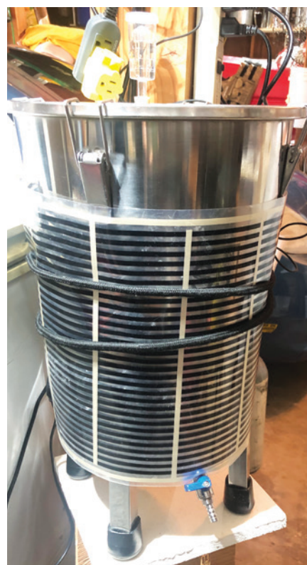
FermWrap™ attached to a temperature controller and secured around the fermenter keeps the fermenter at a set temperature, which is just one of many uses for the heating equipment.
