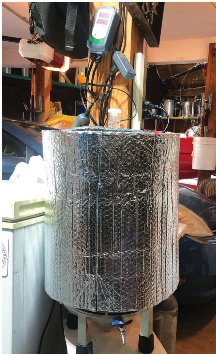
Insulation outside of a heat wrap will hold the heat in and provide even more warmth to the fermenter.
