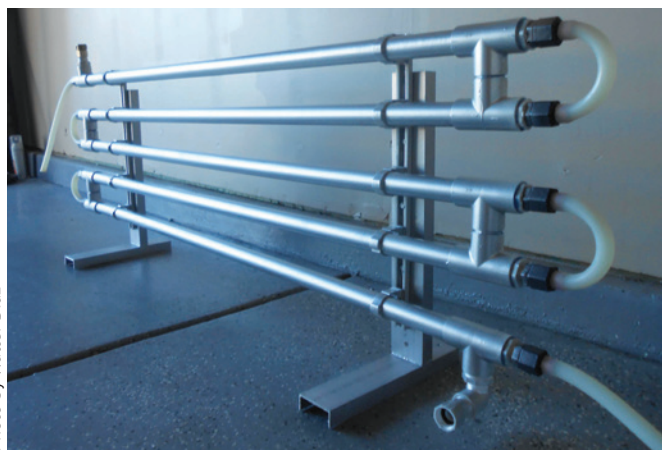
Wort chillers can come in many shapes and forms. This homebrewer-built counterflow chiller has removable end caps so that the interior pipes that the wort flows through can be manually cleaned with a brush.
