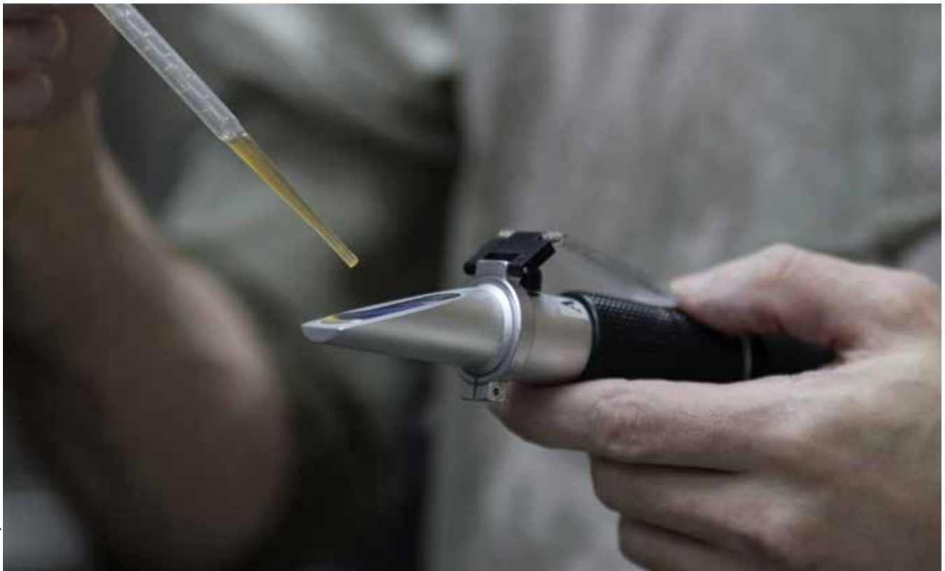
A refractometer can be used to take gravity readings prior to fermentation with just a drop or two of wort.
