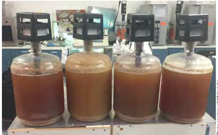
For this temperature experiment the same wort was fermented with the same strain. The two middle carboys were at a higher temperature than two on the outside.
