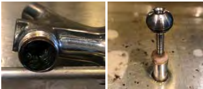
Picture 1 on left and picture 2 on right. The black slime, indicative of Lactobacillus growth seen in picture 1, and the ropey goop found in picture 2, indicating a Pediococcus infection.
