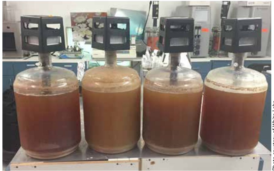
For this temperature experiment the same wort was fermented with the same strain. The two middle carboys were at a higher temperature than two on the outside.
