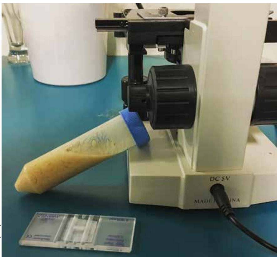
Yeast cell counts can be conducted using a microscope with a 40X objective lens and a methylene blue dye to identify the dead yeast cells.
