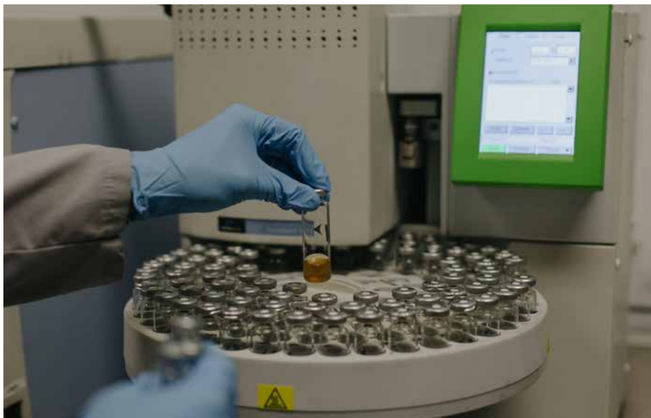
At White Labs, beer samples fermented with different yeast strains are run through a gas chromatograph to quantify some of the aromatic compounds created from the various strains.
