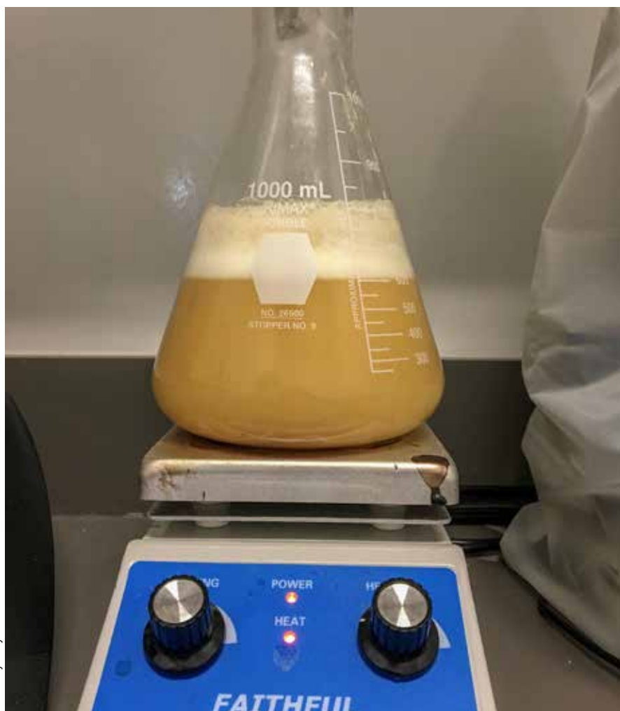
A forced ferment test will show the potential final gravity of a full fermentation within 2–3 days using a heated stir plate.
