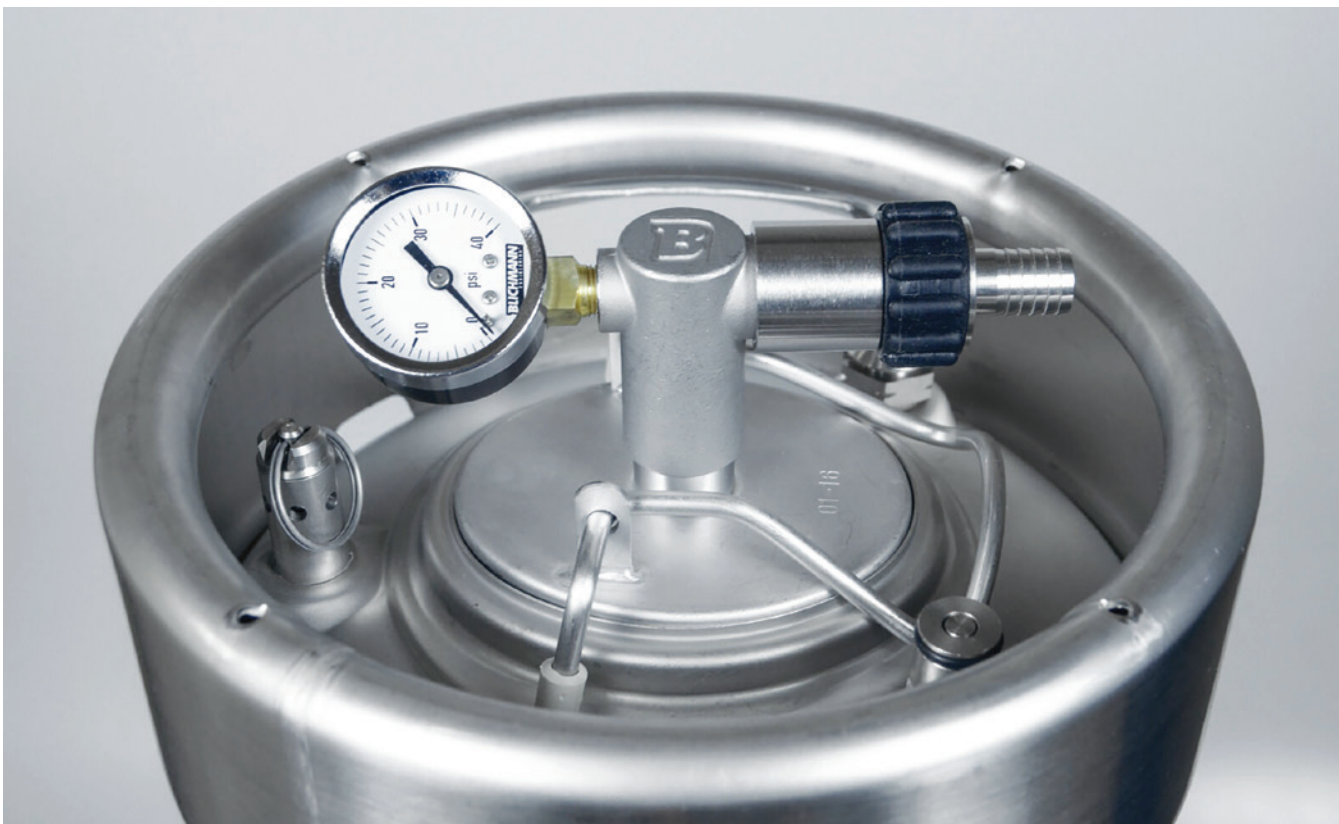
A spunding valve is required to set the pressure you want inside of your fermenter. The valve releases pressure if it builds up over this set amount.
