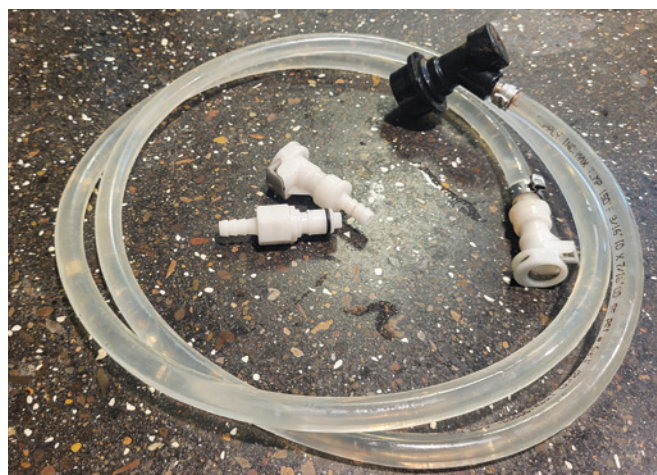
Using John Guest quick disconnects, you can change the length of choker to pour beers at different carbonation levels.
