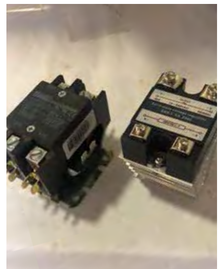
Two common types of switches found in electrical brewing systems. A mechanical contactor is on the left and a solid-state relay with heat sink on the right.
