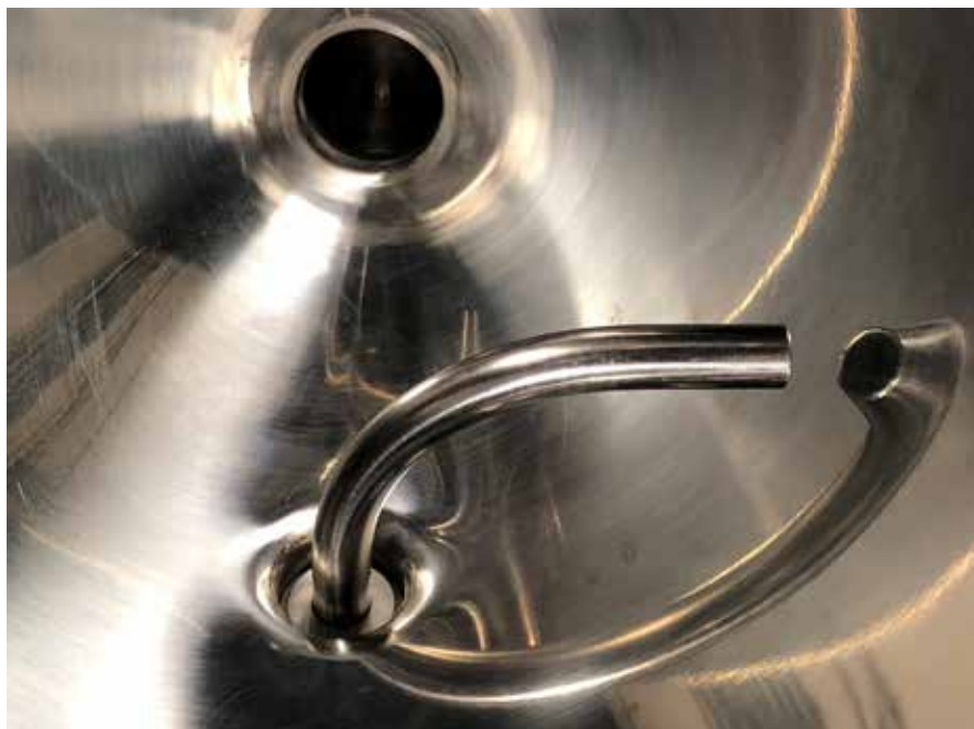
A racking arm is rotated to adjust the level at which beer is transferred from the conical to a keg or bottling bucket, allowing it to be set just above the yeast cake to minimize beer left behind.
