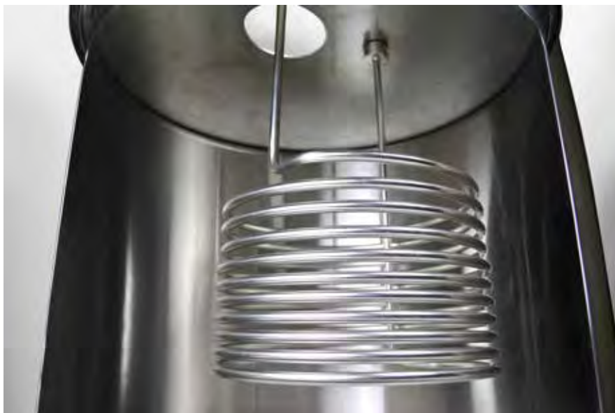
Ice water or glycol can be recirculated through an immersion cooling coil as a way to control temperature inside of a conical. Insulation jackets will help maintain the temperature.
