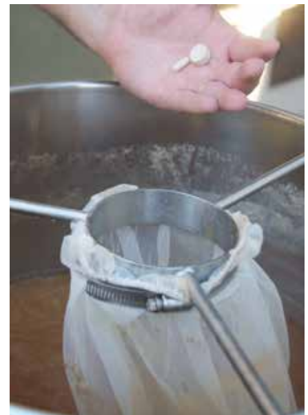
Certain yeast nutrients need to be added to the boil in order to allow their nutrients to be freed up and subsequently assimilated by yeast.
