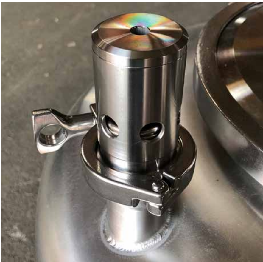
A pressure relief valve is a critical piece of safety equipment to ensure the conical is not over-pressured.
