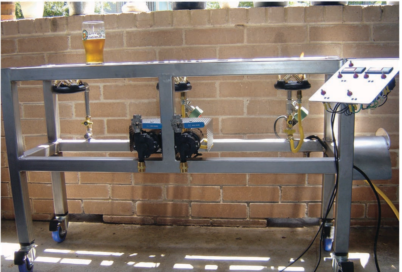
The completed frame, resting on locking casters. This makes it easy to take Brutus "on the road." After this picture was taken, a plate chiller was attached on the lower front beam, on the side opposite the control panel. (See the picture on the front cover.) Note that the burner under the kettle position is manually controlled and lacks the ASCO switch and plumbing of the other two burners. Utilizing a "gas beam" and hiding the wiring in Brutus's frame gives the rig a clean, uncluttered look, but gas lines could be run outside as well.
