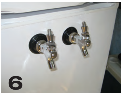
The faucets screw onto the outside of the fridge door. At this point, the hard part is done. You're almost ready to pour beer.
