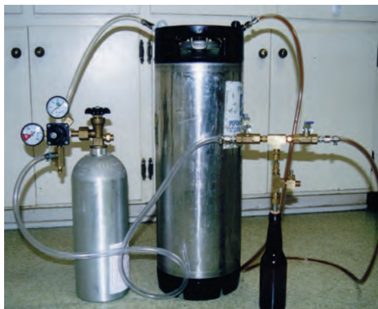
A full set-up for bottling sediment-free beer from a keg — a keg, gas cylinder and counter-pressure bottler.
