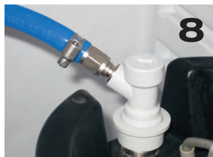
The gas line(s) connect to the keg(s) via the "gas in" post. The first time you apply pressure, you should check for leaks.
