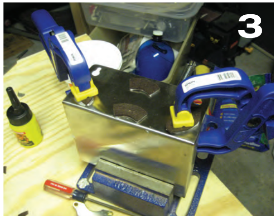
Magnets being glued to the back of a drip tray. This makes removal for cleaning easier. Drip trays can also be bolted into place.
