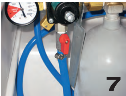
Put your gas line over the barbed fitting on the regulator, and clamp it down. For multiple taps, this line will lead to a splitter.
