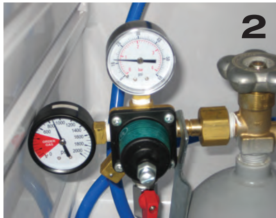
A CO 2 tank with a dual gauge regulator provides the gas to keep the beer carbonated and push it through the lines. For multiple taps, the gas line must be split.
