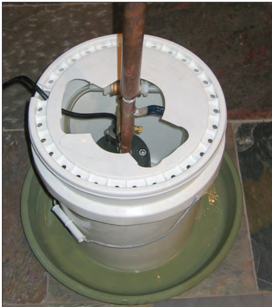
This pumped up bucket project cleans and sanitizes carboys and kegs with ease.
