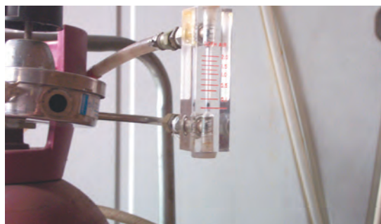
A rotometer measures gas flow through it. Using one can help you fine tune your carbonation levels.
