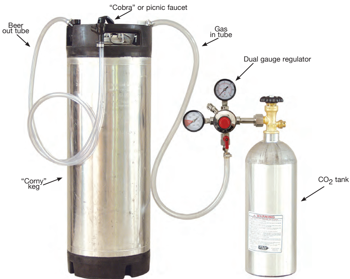
A typical homebrew keggling set up consists of a 5-gallon (19-L) Cornelius keg, 5 lb. (2.3 kg) CO 2 cylinder, regulator with gauges for tank pressure and line pressure, 3/16 ID tubing, posts (partially hidden) and cobra faucet.
