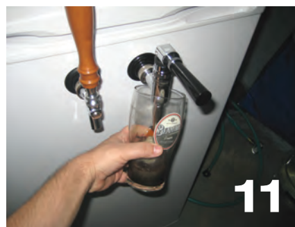
A homebrewed stout being poured from a stout faucet. Pushing beer with nitrogen is another option for this kegerator.
